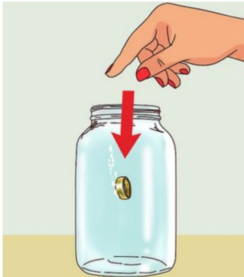
Exact volume will be calculated using the Volume displacement method. Objects will be submerged in a volume of liquid to measure displacement.
