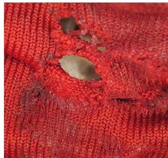
ABRASION HOLES & MOLTEN MATERIAL
