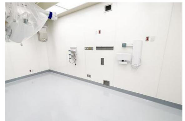
Whiterock is a material commonly used on walls in DNA clean rooms as it provides a smooth and easily cleanable surface.
