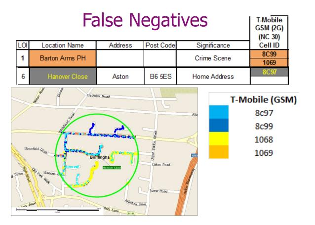
One cell detected as serving at the home address using method #1 Four cells detected serving using method #2
