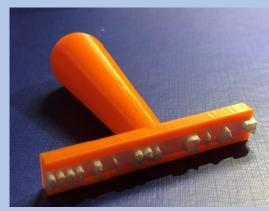
3D printed model adhered to handle
